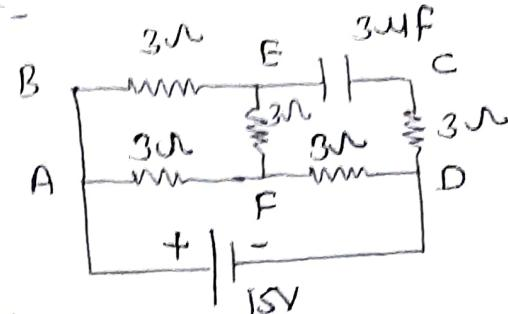
Q1-8: find potential difference between the points A and B for the network shown in figure-
