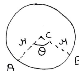
Q:-6: find equivalent Resistance of network shown in figure between points A and B when
